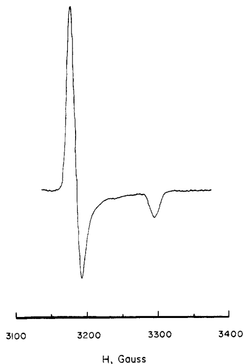
Figure 4. Frozen-solution EPR spectrum of the \text{Ni}^{\text{III}}(\text{CN})_6^{3-} ion at -220^\circ\text{C} and 9.08 GHz.
